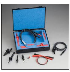
**Model 2187-4 Low Thermal Test Lead Kit:** Includes an input cable with banana terminations, banana extensions, sprung-hook clips, alligator clips, needle probes, and spade lugs to connect the Model 2182A to virtually any DUT. The kit is also used to connect the Model 2182A directly to the Model 622X guard to improve response time for pulsed measurements or to reduce errors when measuring high impedance devices.
