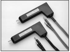
**Model 5807-7 Helical Spring Point Test Leads:** Two excellent Kelvin test probes for Keithley instruments that measure 4-terminal resistance. The probes have pointed tips that rotate when pressure is exerted on the handle. Good contact is assured, and the handle can be held at any angle to the measurement surface. The lead wires terminate in banana plugs. **Lead wire length:** 2m (7 ft).
