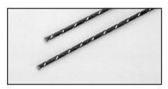
**Model 7401:** Type K thermocouple wire kit includes 30.5m (100 ft) of type K (chromel-alumel) thermocouple wire.
