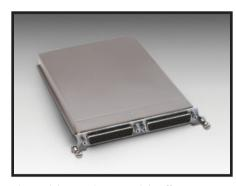
The Model 7703 plug-in module offers 32 channels of 2-pole or 16 channels of 4-pole multiplexer switching that can be configured as two independent banks of multiplexers. The non-latching reed relays provide high speeds and are designed for 300 volt, 500mA; 10VA. The relay closures are stored in onboard memory. The Model 7703 is ideal for RTD and thermistor temperature applications.
