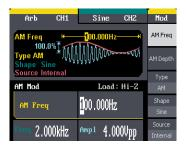
View the modulated waveform on the display and see how it changes when varying the output frequency and carrier waveform.
