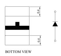
All dimensions are in mm Tolerance: ±0.1mm
