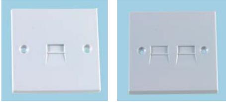
A selection of Master or Secondary (Slave/Extension) wall mounting sockets that are available with IDC or screw terminals. The sockets are either surface or flush mounted and are available in 3 different styles. The master sockets contain a 1.8 $\mu$ F capacitor, whilst the secondary sockets contain terminal connectors only.
