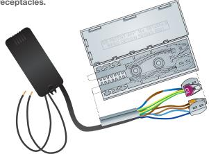
When fitting the cables into the cable clamp the sides of the box need to be eased apart to make an opening. It is normal for the entrance to be splayed apart with the cables in place.
