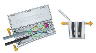
7 Try to keep cables of a similar size together in the same slot and simply push them into the slot as far as they will go.
