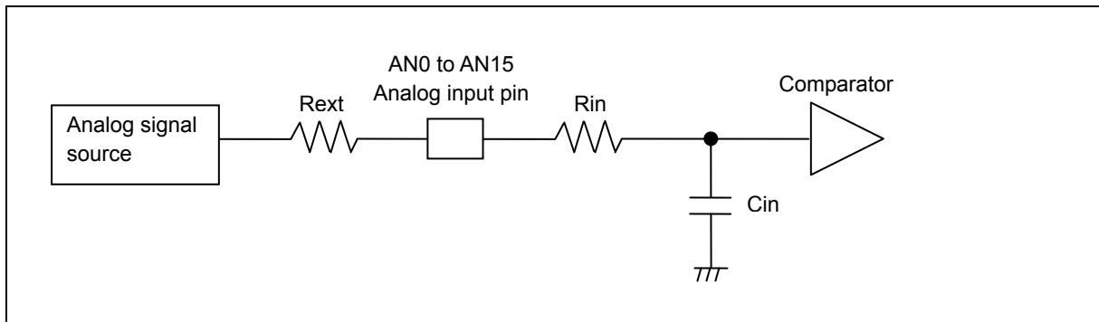
(Equation 1)  $T_s \geq (R_{in} + R_{ext}) \times C_{in} \times 9$
