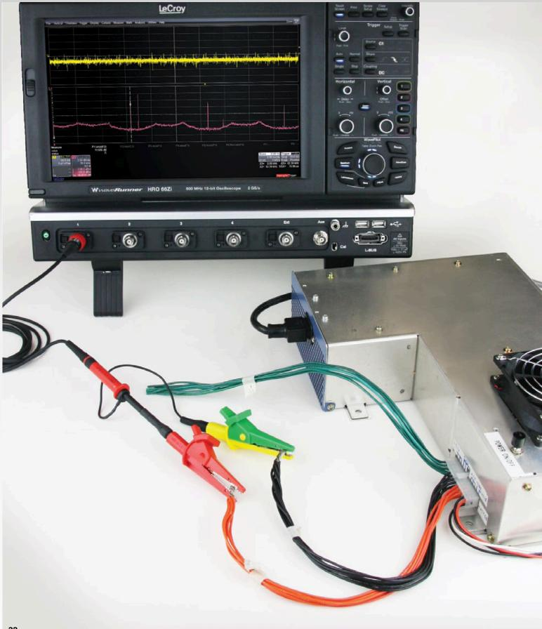
The PPE series of probes are suitable for a wide range of applications where high-voltage measurements must be made safely and accurately. There are five fixed-attenuation probes covering a range from 2 kV to 20 kV, and one switchable probe providing  $\pm 10/\pm 100$  attenuation for voltage inputs up to 1.2 kV.
