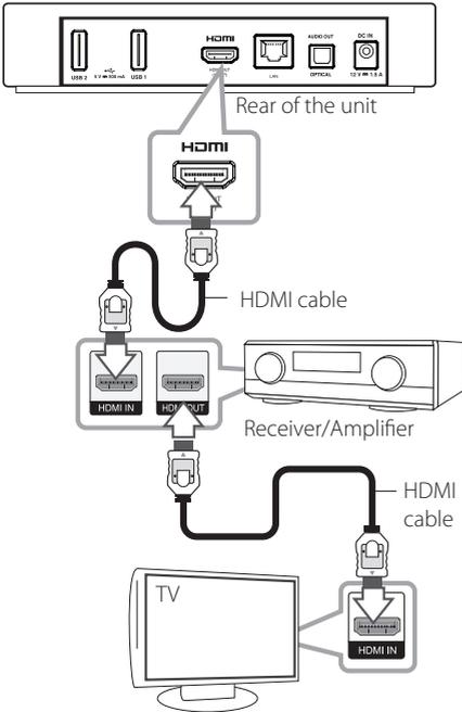
Connect the amplifier's HDMI output jack to HDMI input jack on your TV using a HDMI cable if your amplifier has HDMI output jack.
