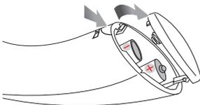
Open the battery cover at the bottom of the Remote Control, and insert two (1.5 V AA) alkaline batteries with **+** and **-** matched correctly.
