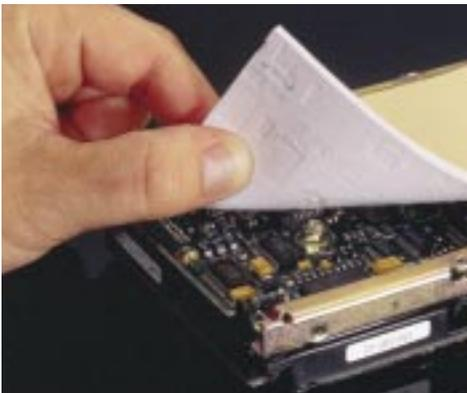
Gap Pad VO is a thermally conductive material that acts as a thermal interface between a heat sink and an electronic device. The conformable nature of Gap Pad VO allows the pad to fill in air gaps between PC boards and heat sinks or a metal chassis.
