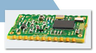
High-performance, long-range radio module with embedded M-Bus protocol, for data exchange in stationary and mobile systems between gas, water, heat, electricity meters and concentrators.
