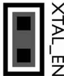
Figure 6-21: External Crystal Circuitry Enable (CT4)
