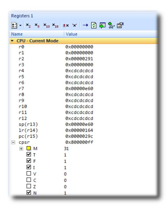
There are four register windows, so you can open and display four sets of CPU and peripheral registers at the same time. You can configure which registers and peripherals to display in the **Registers** windows individually. As you single-step the program, the contents of the **Registers** window updates and any change in a register value is highlighted in red.
