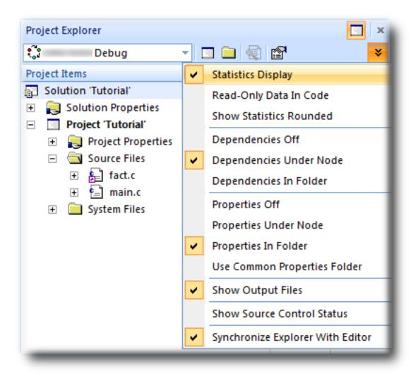
When the **Statistics Column** option is checked, the **Project Explorer** displays two additional columns, **Code** and **Data**.
