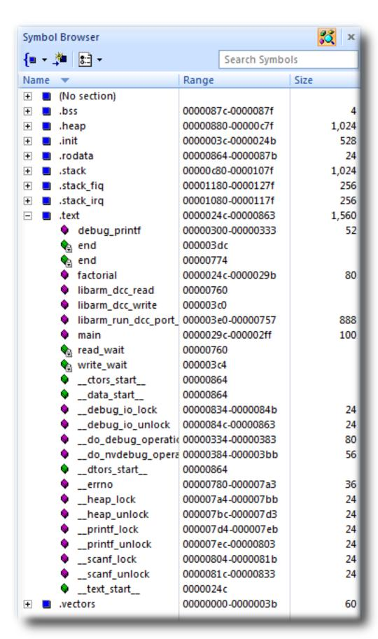
Here, we can see that **main** is 100 bytes in size and is placed in memory between addresses 0000029C and 000002FF, inclusive, and that **factorial** is 80 bytes and occupies addresses 0000024C through 0000029B. Just as in the **Project Explorer**, if you double-click a function, CrossStudio moves the cursor to the line containing the definition of that function, so you can easily use the **Symbol Browser** to navigate around your application.
