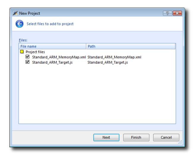
The **Project files** group shows the files that will be copied into the project. The only files used are the memory map file, which describes the memory layout used by the application, and the script used to reset and control the target. For the debugging session to work correctly, each of these files must match and be appropriate for the application you are debugging.
