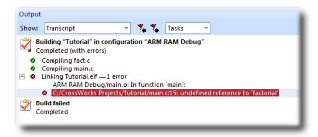
The remaining error is a linkage error. Double-click fact.c in the **Project Explorer** to open it for editing and change the two occurrences of fact to factorial. Rebuild the project—this time, the project compiles correctly:
