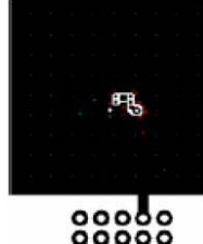
b) 173 °C/W when mounted on a minimum pad of 2 oz copper.
