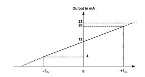
Note: 1) The performance specified in the datasheet is valid within the 4-20 mA output range only.
