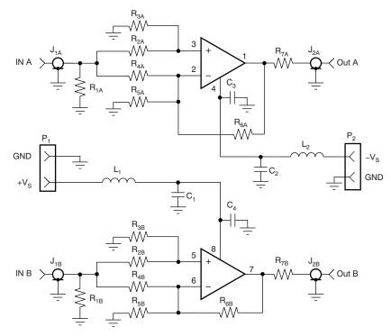
Figure 2. Schematic for DEM-OPA-SOT-2A
