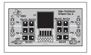
Figure 3. PCB Layout - Top Assembly
