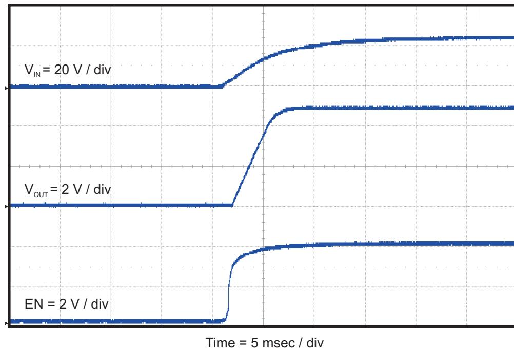
Figure 9. TPS5401EVM-708 Start-Up Relative to  $V_{IN}$
