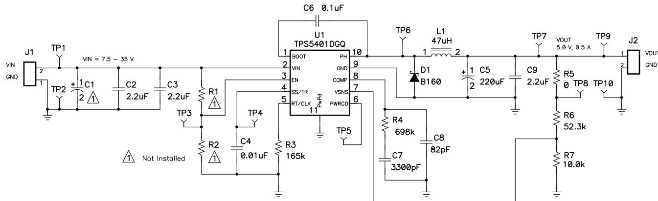
**Figure 14. TPS5401EVM-708 Schematic**
