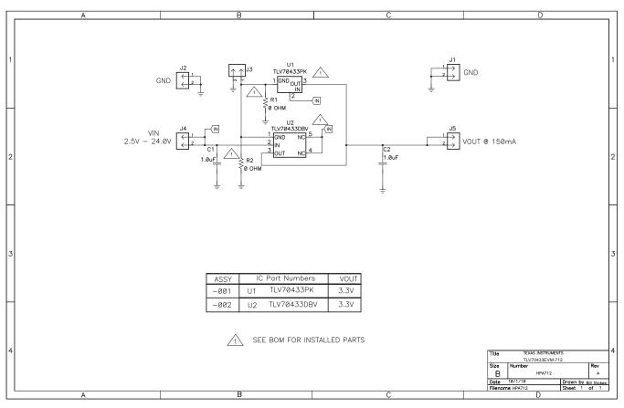
Figure 6. TLV70433DBVEVM-712, TLV70433PKEVM-712 Schematic
