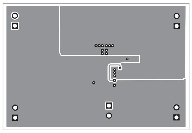
Figure 5. Bottom Layer Routing
