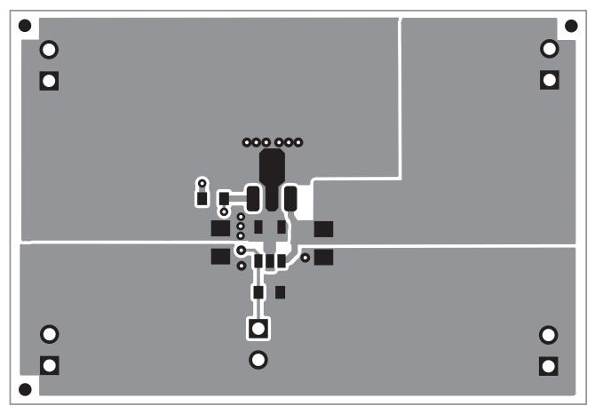
Figure 4. Top Layer Routing
