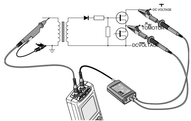
Note that the timing circuit for the FET (Field Effect Transistor) drive is referenced to earth ground. The gate drive signal is isolated with a transformer coupling to the FET, which is connected to the DC-voltage.
