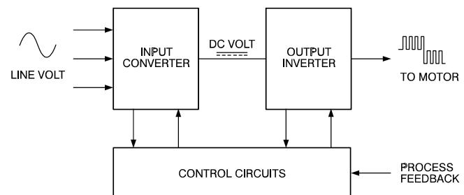
When one of the stages of the output inverter does not function properly, check the following:
