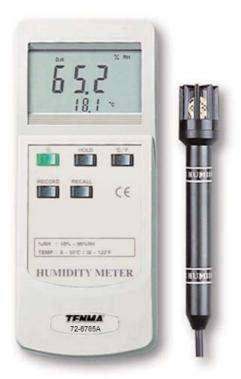
Wide measurement range of both RH and temperature. Humidity measurement uses a high precision thin-film capacitance sensor for fast response. Thermistor sensor for fast response temperature mesurement. Includes instruction manual and probe. Requires 9V battery (not included).
