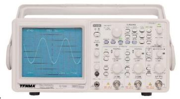
Type 72-7230 oscilloscope offers a combination of analog and digital acquisition modes. Giving you the best of both worlds. Select analog mode when true real-time acquisition is needed and digital mode when pre-trigger events need to be seen. Select save and recall waveforms or freeze transients that are impossible to see with an analog-only scope.
