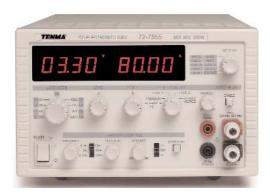
Type **72-7855** compact electronic DC load is ideal for testing a wide variety of DC power sources. It can be used to investigate the behavior of many different types of power sources such as batteries, solar cells, fuel cells, as well as electronic power supply units. Type **72-7855** can operate at voltages below 500 mV for currents up to 10A. This low operating voltage allows it to be used for many low voltage applications. Includes power lead and instruction manual.
