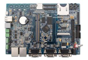
MBS-SAM9G25 SBC board operates at up to 400MHz, with 256 Mbytes NandFash ,128MB DDR II,4MB serial DataFlash and 64KB serial EEPROM. It supports Linux 2.6.39 ,offer angstrom and android-2.3.5\_r1 test .The board provides a wide range of peripherals, including a high-speed USB2.0 port(480MHz), an Ethernet 10/100M interface, audio interface, a JTAG debug port,Micro SD card interface,SD/MMC card interface, CMOS camera interface.It supports video data collection.
