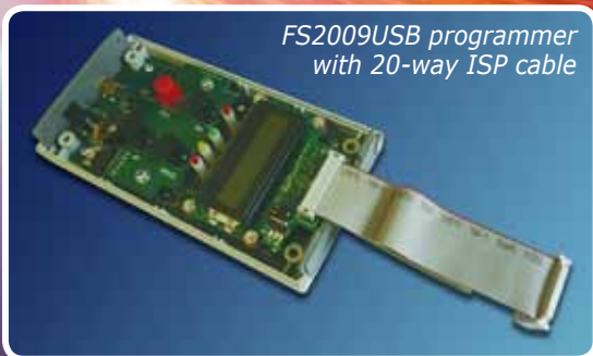
The FS2009USB ARM programmer being used in standalone mode
