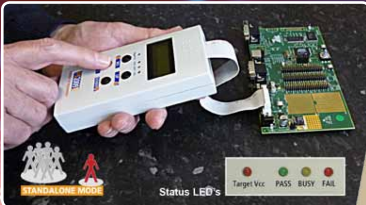
The FS2009USB ARM programmer being used in standalone mode
