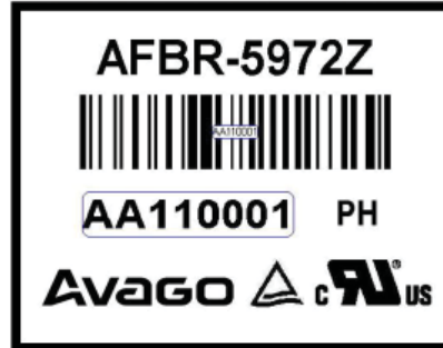
Figure 12. The AFBR-5972Z product label contains lot, year, work week and serial number and country of origin information
