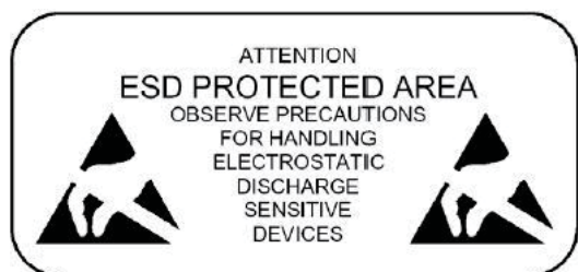
Figure 10. Warning sign for an ESD protected area
