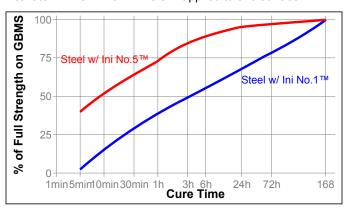
The graph below shows the shear strength developed with time on PVC lap shears and tested according to ISO 4587 Activator Ini No.1™ or Ini No.5™ applied to one surface
