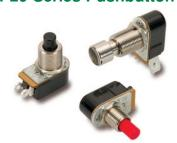
The P26-Series pushbutton switches are single pole, AC rated for 8 amps at 125 VAC and suitable for shallow back Electrical Life panel applications. These switches are momentary action with a medium actuation force (13 oz. typical). The P26-Series switch is equipped with a slow-make, slow-break 100,000 cycles contact mechanism. Typical applications include usage for an Alarm or Warning Device, as well as Test and Measurement Equipment.
