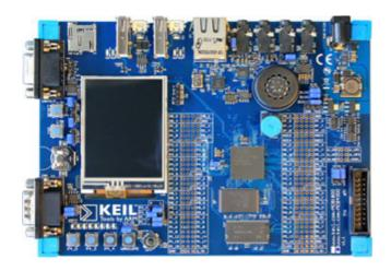
The Keil MCB1800 Evaluation Boards enable you to create and test working programs based on the NXP LPC1850 family of ARM Cortex<sup>TM</sup>-M3 processor-based devices.
