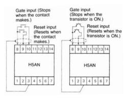
When connecting a solid-state circuit not of the open collector type to the gate or reset inputs as shown below, the voltage of the solid-state circuit (+V) should be 13 to 30 V, and the  $V_{\text{CE(S)}}$  of the transistor should be less than 3 V (the current that flows from either terminal 9 or 10 is approximately 10 mA). Moreover, it is essential that the circuit be ON for gate or reset input, and OFF when there is no input.
