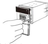
The internal unit comes out by loosening the internal unit fixing screw.
