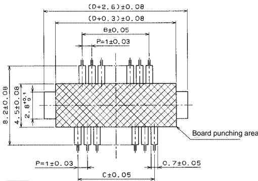
Note : The shaded area indicates the through-hole area.
