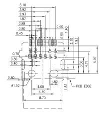
RECOMMENDED PADS LAYOUT (TOP VIEW>SCALE 4:1 NOTE:TOLERANCE FOR PCB LAYOUT IS ±0.05
