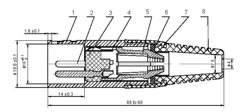
The pin plating silver, thickness 0.5µm (SOLDER).
