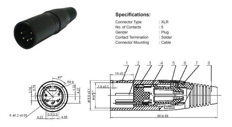
The pin plating silver, thickness 0.5µm (SOLDER).
