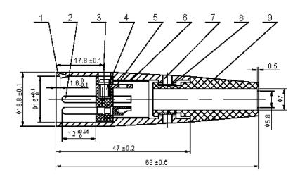
The pin plating silver, thickness 0.5µm (SOLDER).
