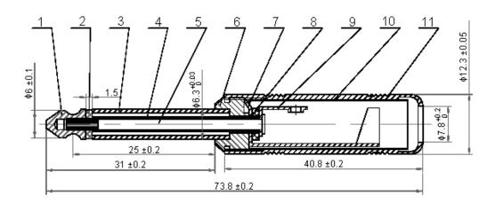
The terminal plating silver, thickness 0.5µm (SOLDER).
