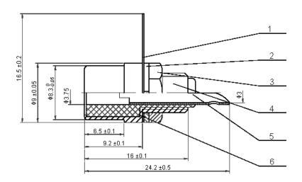
The female pin plating nickel, thickness 1µm (SOLDER).
