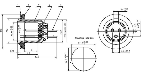
The pin plating gold, thickness 0.05µm (SOLDER).
