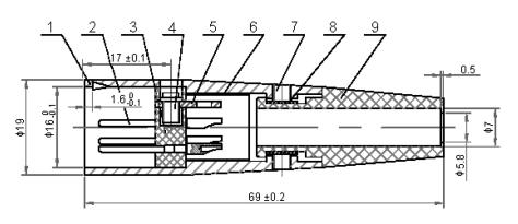
The pin plating silver, thickness 0.5µm (SOLDER).
