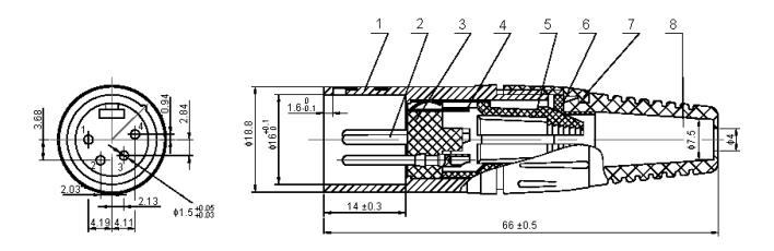
The pin plating silver, thickness 0.5µm (SOLDER).
