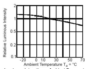
Luminous Intensity vs. Ambient Temperature
