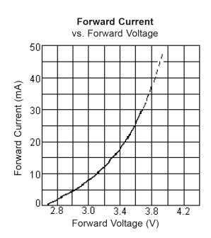
White Typical Electrical Optical Characteristics Curves  $(T_a = 25^{\circ}C \text{ Ambient Temperature Unless Otherwise Noted})$
