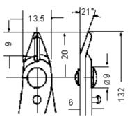
Cutting Capacity : 14 AWG (11.6 mm)
