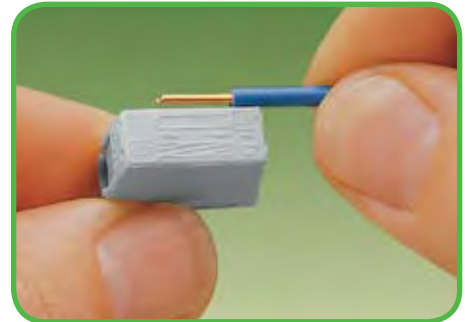
Strip conductor to 9 – 11 mm / 0.39 in
