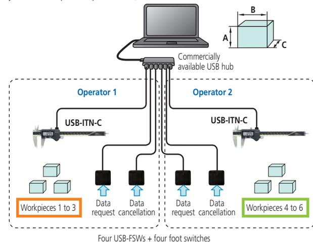
Because multiple operators are making measurements in parallel, the operation buttons in the following window and function keys, of which the system has only one, cannot be used. Only foot switches, for which multiple measuring instruments can be used, are available (by way of USB-FSW).
