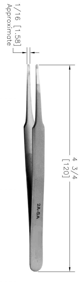
Material: Anti-Magnetic, Anti-Acid, Stainless Steel Style: 2A-SA
