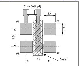
To maintain stable operation, provide a 0.01uF to 0.1uF by-pass capacitor at a location as near as possible to the power source terminal of the crystal product (between Vcc - GND).
