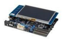
The SAM9N12-EK Evaluation Kit enables rapid evaluation and code development of applications running on a SAM9N12 device.
