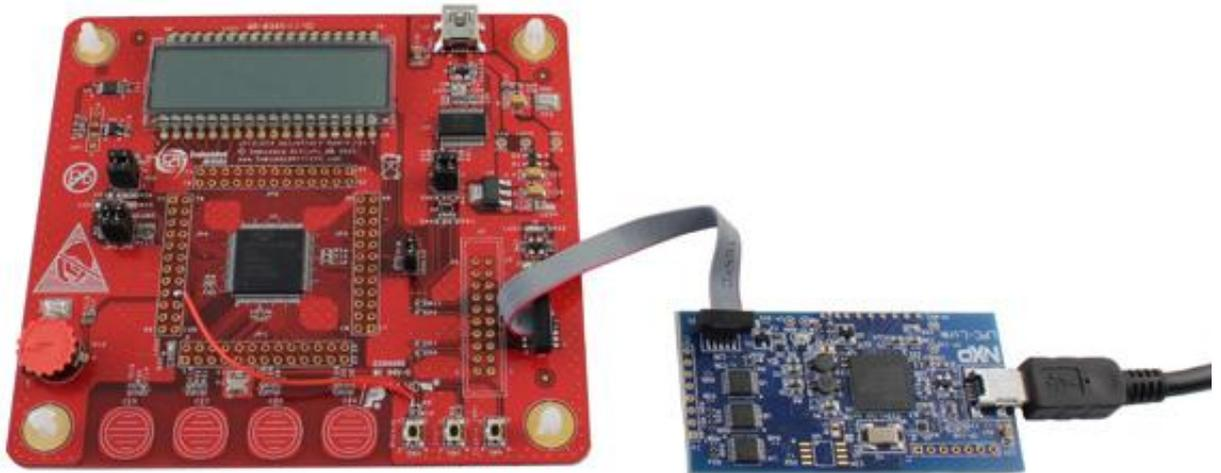
Figure 8 – LPC11D14 QuickStart Board connected to LPC-LINK, via SWD
