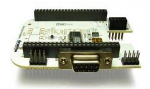
The BeagleBone CANBus Cape makes use of DCAN1 interface of the AM335x processor. The CAN Bus interface can be accessed via a standard D-Sub 9 female serial connector. This connector is located to the side so it doesn't interfere with any capes stacked above it. The BeagleBone CANBus Cape will support SocketCAN.
