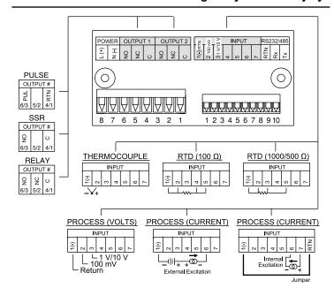
Connect the main power connections as shown in the figure below.
