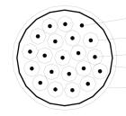
GROUND;7x 0.16mm TIN PLATED Cu INNER JACKET:20x 1.0mmPVC INNER CONDUCTOR:20x9/0.1mmCU SCREENING: 20x0.025mmAL OUTER JACKET: 08.5mmPVC BLACK
